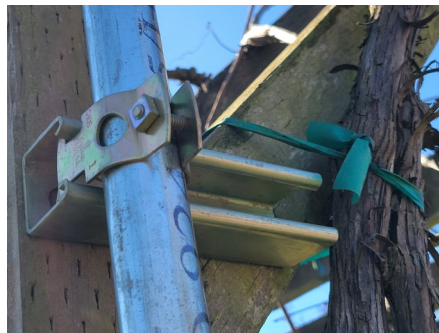
Mounting mechanism to mount pipe to fence post.
